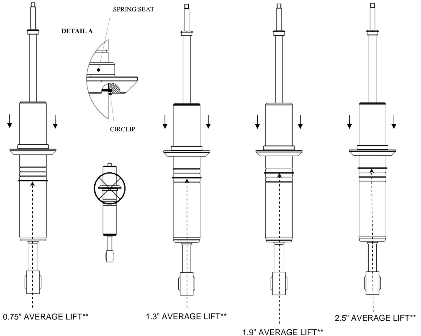
\*\* Ride heights indicated are typical. Actual ride height is influenced by which factory suspension the vehicle is equipped with and its condition; optional equipment and accessories on your vehicle, and other vehicle modifications such as replacement coil springs, wheel and tire combinations, etc.
