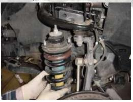
12. Position the new coilover onto the vehicle, sliding the top into the shock tower first. Install the top three nuts which hold the coilover to the shock tower finger tight. Install the lower shock bolt and nut. You may need to pry down on the upper control arm in order to get the lower shock bolt installed. Torque upper nuts and lower bolt/nut to manufacture specs.
