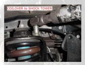
11. Being careful not to overextend and pull apart the inner CV Axle joint, move the spindle/hub assembly out of the way so the coilover can be removed from the vehicle. Remove the coilover on both sides.
